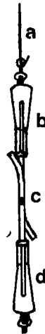
FIGURE 5 Breaking apparatus for parallel-axis bonds: (a) hook connected to Instron load cell, (b) upper spring clamp, (c) parallel-axis bond pair, (d) lower spring clamp connected to Instron load cell.
