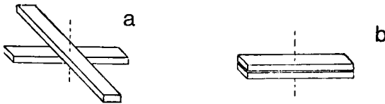
FIGURE 1 Fiber arrangements for laser bonding of rectangular monofilaments: (a) crossed fibers, (b) parallel fibers.
