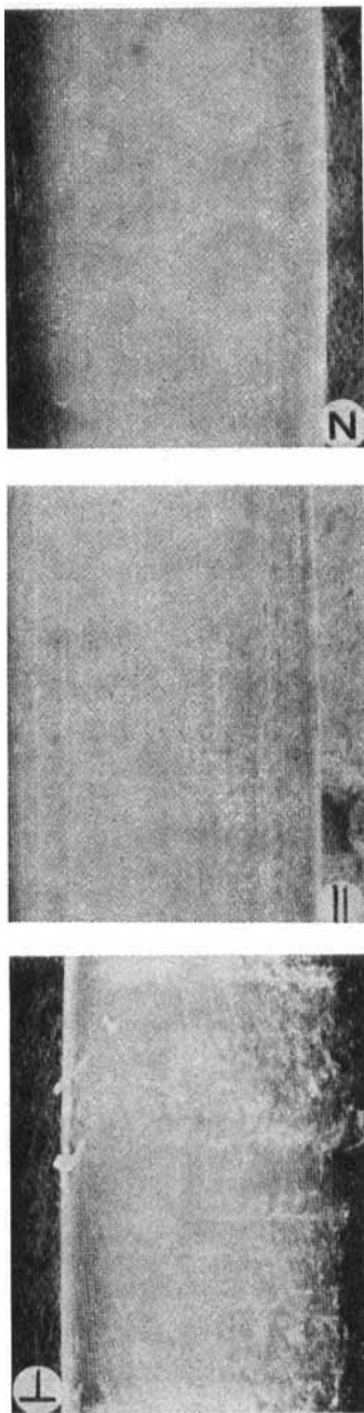
FIGURE 6 Scanning electron micrographs ( \times 100 ) of monofilament surfaces: original nominal scratches, N; parallel scratched, ||; perpendicularly scratched, \perp .
